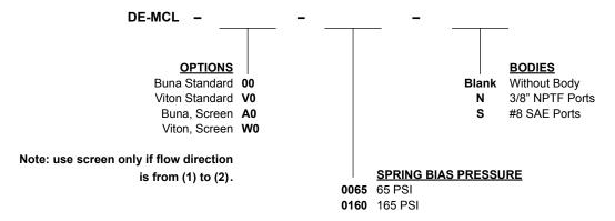
Note: pressure above SPRING BIAS PRESSURE at port (2) may cause valve to self open.
