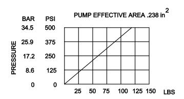
FORCE ABOVE CURVE IS WITH HYDRAULIC OIL 150 SSU AT 100°F.
